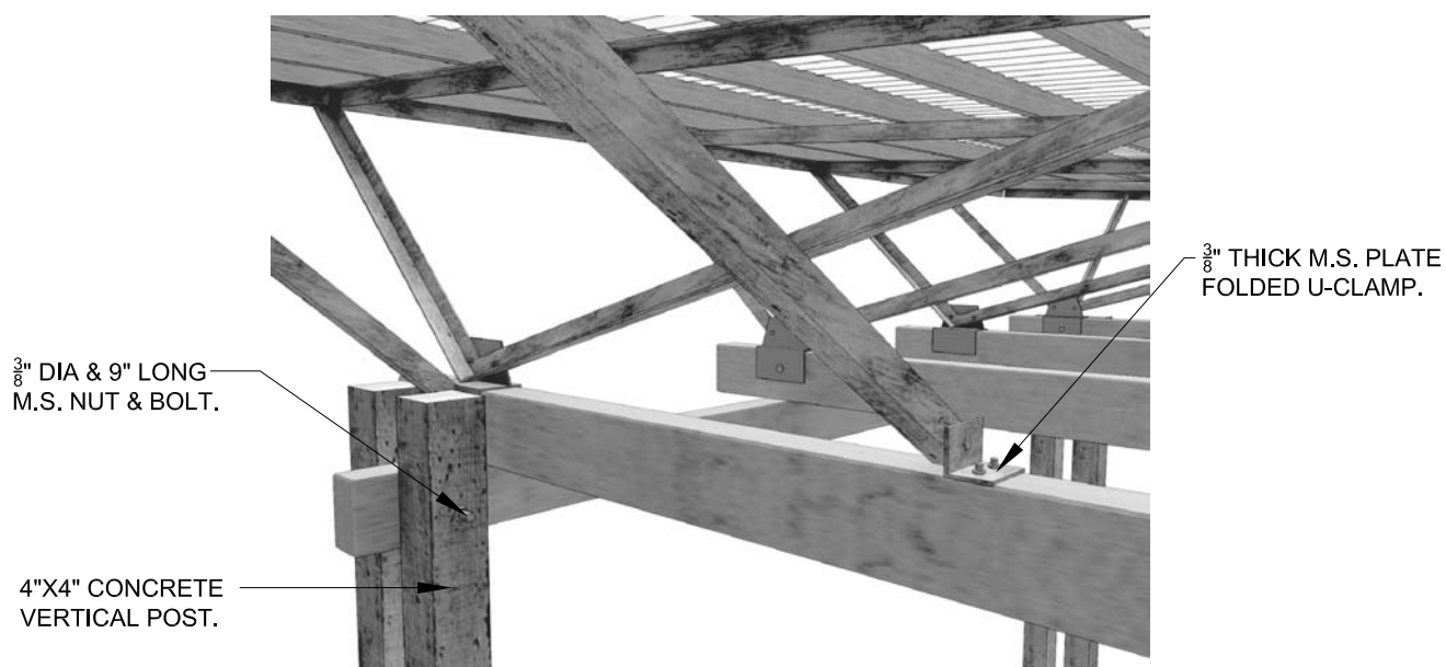
DETAIL OF ROOF FRAME
