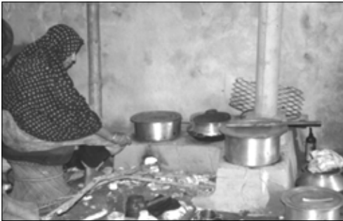
Stove near Chunati WS in 2007. Note concrete chimney tube for exhaust. Danger to children in use of metal exhaust pipes, and easy access to concrete, brought on this adaptation. [Philip J. DeCosse]
