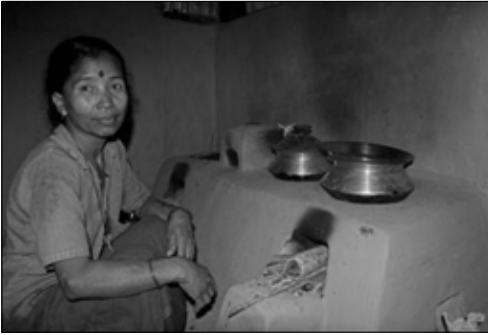
Nishorgo-supported stove in 2008. Smoke exhaust goes out by this time through the back wall. [Sirajul Hossain]
